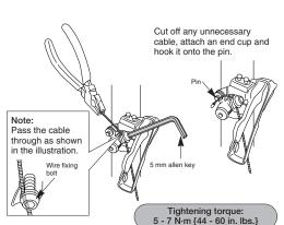
After taking up the initial slack in the cable, re-secure to the
