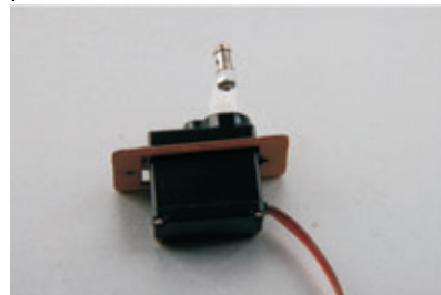
8. Install the servo into the servo mount.
