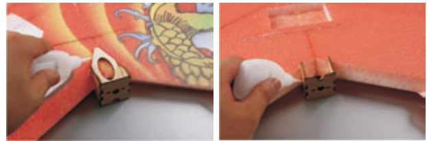
4. Install the motor mount by using CA, pls make sure to paste flatly, can not be bend up and down, if bend, will affect the motor thrust wire, and also affect the flying performance.
