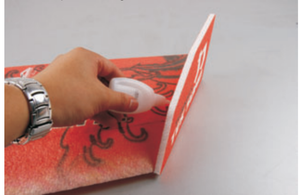
23.Glue the two wing fences by using CA.
