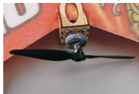
24.Fix the propeller by using O-ring.
