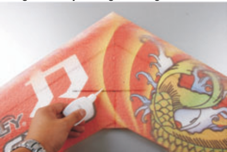
3. Put another carbon rods into the pre-cut slot of the front wing by using CA to glue.
