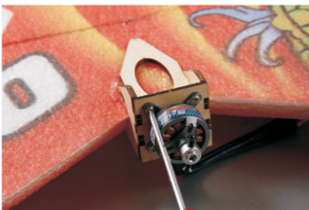
16. Install the motor by using the self-tapping screws which included into the motor parts bag.
