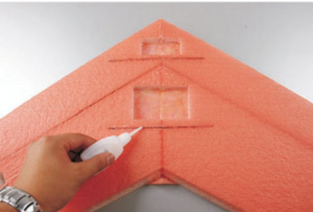
2. Put 2 pcs carbon rods into the pre-cut slots of the wing back by using CA to glue
