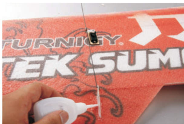
13. Using the CA to glue the control horn.
