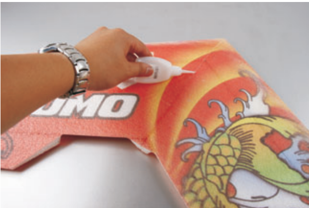
1. Glue the left and right wing by using CA glue, must be working in a flat surface, to ensure the two wings can not be distortion.
