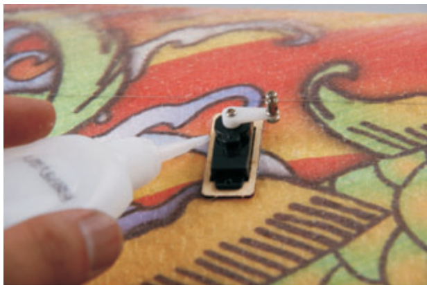
9. Install the servo onto the pre-cut servo hole as the picture shown , by using the CA to glue .
