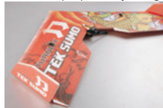
25.Pls make sure to adjust the CG ( 200-212mm ) of the flying wing before fly it , because the CG is very improtant to the flying wing.
