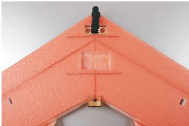
6. Thread the plastic band through the pre-cut hole of the wing.
