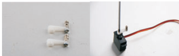
7. Install the pushrod connector onto the first hole of the servo arm, and then install the servo arm onto the servo, pls make sure the servo arm is in the neutral position.
