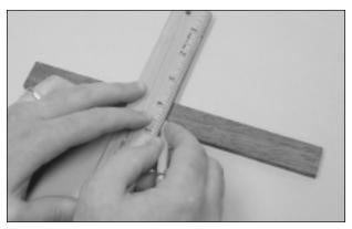
☐ Use a ruler and a pencil to locate and draw a vertical centerline on each side of the hardwood wing joiner.
