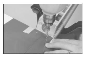
☐ Using an 11/64" diameter drill bit, drill two holes into the wing and through the plywood wing hold-down block inside the fuselage. Locate one hole in each wing panel, 3/4" out from the centerline and 1/2" in front of the trailing edge.
