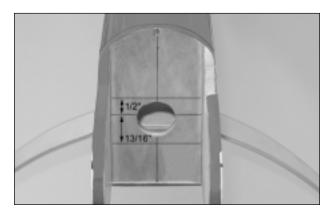
☐ Using a ruler and a pencil, measure and draw one horizontal line 1/2" **above** the horizontal centerline and one horizontal line 13/16" **below** the horizontal centerline.
