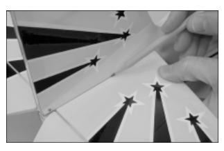
☐ When satisfied with the fit and alignment, use a pencil to draw a line on each side of the stabilizer where it meets the fuselage sides. Do this on both the top and the bottom.
