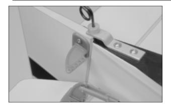
☐ Install one control horn onto the left side of the rudder, making sure that the centerline of the control horn is 1/2" up from the bottom of the rudder (at the hinge line), and that the front edge of the control horn is perpendicular to the rudder hinge line.
