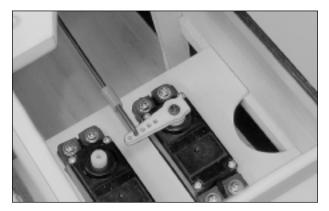
☐ Using a pair of pliers, carefully bend the pushrod wire down at a 90° angle and cut off the excess, leaving 5/16" of wire beyond the bend.
