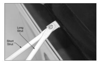
☐ Install one long strut and one short strut to one side of the mounting strap, using one M3 x 8 machine screw, one M3 flat washer and one M3 hex nut.
