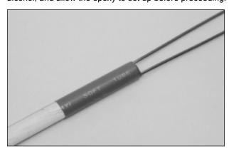
☐ Slide one piece of heat-shrink tubing over each end of the dowel and use a heat gun to shrink the tubing.
