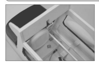
☐ To secure the fuel tank into position, apply a bead of silicone sealant around the joint between the back of the fuel tank and the forward bulkhead.
