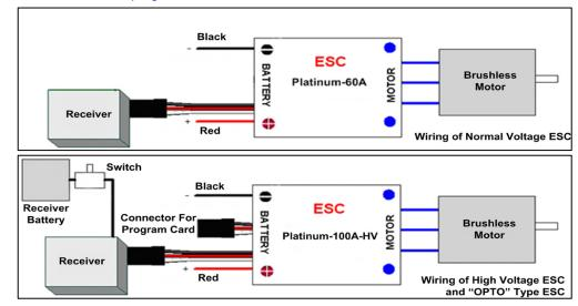
There is a thin black wire attached with the negative input wire (black color, thick) of the ESC of Platinum-150A-OPTO, Platinum-70A-HV, Platinum-120A-HV, it is used to eliminate the spark when the battery pack is connecting with the ESC. Please use it in the following sequence:
