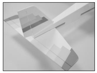
□ Glue the stab and fin to the fuselage with epoxy, keeping the stab and fin in position as diagram shown.
