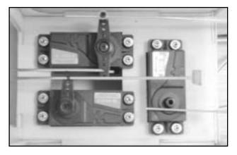
□ Now it is time to hook the servos up to the control surfaces. Using Z-bend pliers, makes a Z-bend at the marked location. Cut off the excess rod. Insert the Z-bend into the servo arm .
