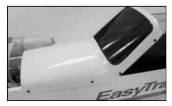
□ Put the windshield on the front fuselage. It is held in place with eight  $2 \times 5$  wood screws. You will need to drill a 1/16" pilot hole for each screw first. Glue the window onto the windshield with CA.
