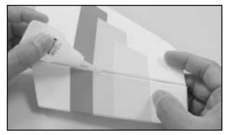
□ Remove the elevator and rudder and glue the hinges into the control surfaces using the same technique outlined for the ailerons.
