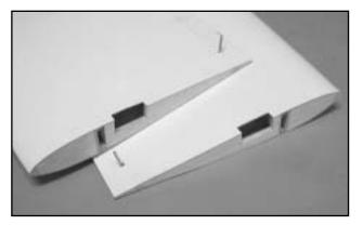
□ Also remove the portion of center wing rib in this area to allow clearance for aileron servo. Repeat the same process on the other wing half.
