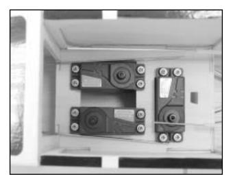
□ Mount three servos on the servo tray which is already installed in your fuselage. Note their orientation in the photo. Follow your radio's instruction manual and make sure you use the grommets, eyelets, and screws furnished with your radio. Drill 1/16" pilot holes for the mounting screws before insertion.
