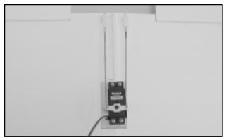
□ Hookup to the ailerons is via a nylon horn that is threaded onto the torque rod that is already installed in the wing. Screw the horn down until there is about 1/16" of threads exposed above the horn. Use threaded rods with clevises on the end for the linkage. Bend a "z" bend on the servo end of the rod at the proper length so you have neutral aileron when the servo is centered.
