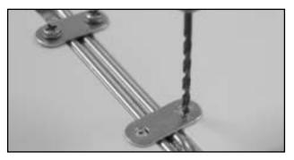
□ Position the two metal landing gear straps across the landing gear struct. Using a felt tipped pen, mark the location for the four landing gear mounting strap holes. Drill the four mouting holes as marked with 3/32" drill bit. Secure the mounting strap by four 3 x10 screws.
