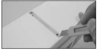
❑ Locate the main landing gear channel in the bottom of the fuselage. Use a sharp hobby knife to remove any covering from the slot. You might lightly coat the exposed wood in the landing gear slot with 5-minute Epoxy to prevent the wood from becoming fuel soaked.
