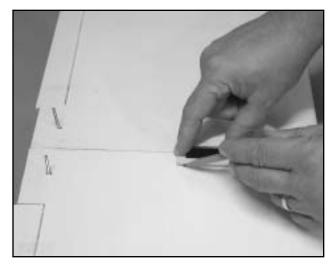
□ Place the servo tray centered over the cutout in the bottom of the wing. Mark around the servo tray with a pencil.
