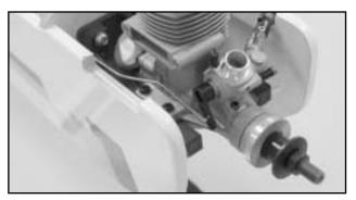
□ Using either Z-bend pliers or a regular pair of pliers, make a "Z" bend in one end of one .050" piece of wire. Slide it into the throttle linkage tube.
