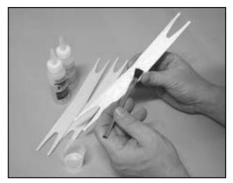
□ Mix up some 5-minute epoxy and apply it to both sides of one of the joiners. Sandwich this piece between the other two joiners and align the edges of all three joiners.
