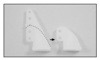
□ Cut the control horn as photo shown.
