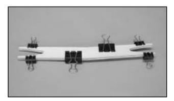
□ Clamp the three joiners together with clothespins or other small clamps and wipe off the excess epoxy before it cures. Allow the epoxy to cure before removing the clamps.
