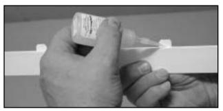
□ To hinge the ailerons, remove the clear tape that holds one of the ailerons in place. Pull the aileron off the wing, revealing four hinges. Center these hinges in their slots in the AILERON and secure them with <u>THIN</u> CA, letting it wick into the joint. Glue both sides of the hinge.
