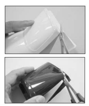
□ Locate the windshield and window. Trim the windshield and window along with the molded cutting line with curved scissors.
