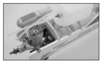
□ Attach a 6" piece of standard fuel line (not furnished) to both the fuel outlet nipple and the vent nipple on the tank.
