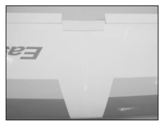
□ Locate the white trim tape and apply to center wing joint. Start at the servo tray and work around the wing. Gently pull on the tape while pressing it down onto the wing to slightly stretch the tape into place and provide a smooth seam. You will have to use Heat Iron to iron the trim tape if you have Ultracote covered Trainer.
