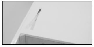
□ Same way to the nosegear tubing. You will have to use hobby knife to cut away the covering then insert the tube through the first former and second former.
