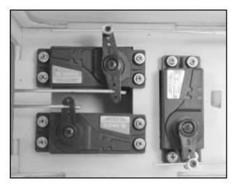
□ Install the pushrod connector onto the outermost hole in the rudder servo arm and throttle servo arm as shown.
