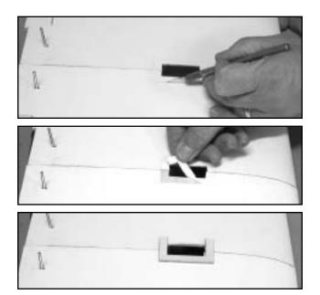
□ Remove the tray, and use a sharp knife to score the covering material where marked. Remove the covering material to expose the wood underneath. Use thick CA or epoxy to glue the servo tray securely in place.
