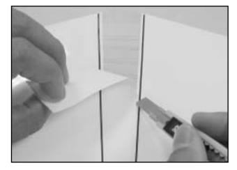
□ Remove the stab and fin from the fuselage and use a hobby knife to carefully score the covering material where marked. Make the score approximately 1/16" inside the lines you drew. It is very important that you do not press hard enough to cut into the wood itself or the stabilizer may fail in flight. Just score the covering and it will peel away nicely.
