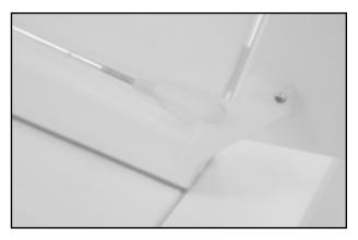
□ Locate the control horns and 2x12mm screws. Snap the clevis onto the control horns. Now position this horn onto the Rudder in such a way that the nyrod runs straight and the holes in the control horn are in line with the hinge line of the stabilizer. Mark the location of the control horn mounting holes on the elevator. Next, drill 5/64" holes where marked.
