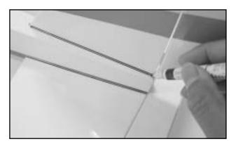
□ Use ruler to decide the center of stab and make marks. With the main wing centered on the fuselage, position the horizontal stab first then you can see the marks you drew through the slot. Then, position vertical fin. Use a felt tip pen or marker to draw lines along the fueslage sides. Do not forget draw lines at the bottom side of stab.
