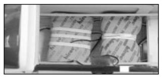
❑ Wrap your receiver and battery with packing foam which is available at local hobby shop. Install the receiver and battery in the front of the servo tray. Receiver is near the servo tray and battery is far from the servo tray as shown.
