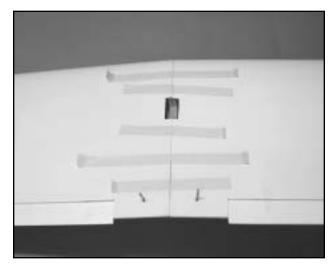
□ With 30 minute epoxy, liberally coat all sides and edges of the wing joiner and slip it into one wing half. Now coat the inside edge of the center wing rib where it will join to the other wing half. This is called the "root" of the wing.
