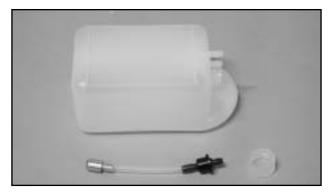
□ Assemble the fuel tank by first cutting the silicone tube to 2-1/2" in length. Press the straight plastic nipple (the 90 degree nipple is not used in this plane) into the rubber stopper (Saliva will ease insertion.) Now slip the silicone tubing onto the nipple and insert the metal clunk into the other end of the tubing. Insert this assembly into the tank (clunk first) and securely tighten the threaded cap on to hold everything together.
