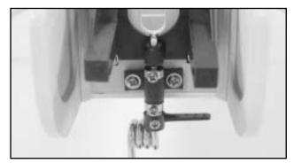
□ Attach the engine mount plate, both mounting beams and the nose gear bearing to the fire wall using the 6-32 x 18mm screws provided. Make sure the mounting beam "webs" are near the outside of the mount. It is not necessary to fully
