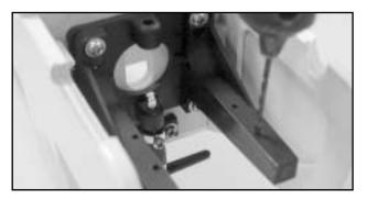
□ Remove the engine and drill a 3/32" hole at each of the four marks you just made. "Breakin" the mounting holes by inserting a 3 x 15mm sheet metal screw into each hole without the engine in place. A drop of oil in each hole may help the screws thread in easier.
