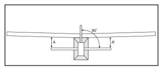
The fin is perpenducular to the stab. Both stab tips to the main wing are equal from the rear view (A=A')
