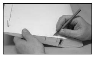
□ On the bottom of one wing half, make a mark 3/8" (10mm) from the inside edge of the wing, between the pre-cut slot in the center rib and the rear edge of the spar box. Use a hobby knife to cut away the covering and balsa sheeting in this area.
