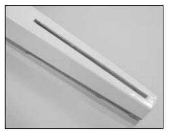
□ Trim away the covering from the slot at the rear of fuselage where vertical fin and horizontal stab go.
