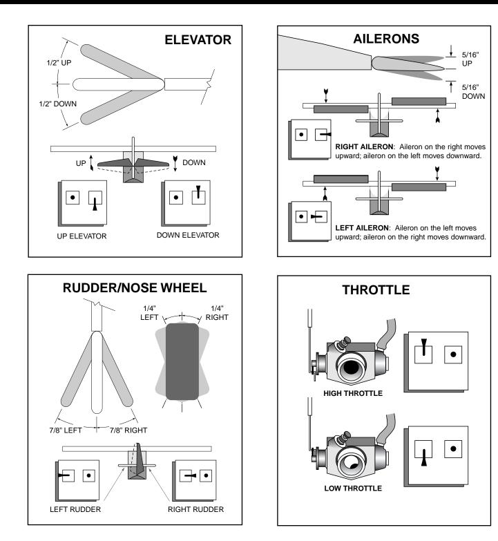
□ Adjust the linkages so you get the proper amount and direction of control throws as illustrated. To INCREASE the amount of movement, move the linkage outward on the servo arm OR inward on the control horn. To DECREASE the amount of movement, move the linkage inward on the servo arm OR outward on the control horn.
