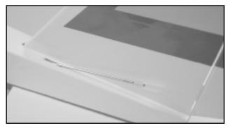
□ Remove the covering on the slot. The rudder and elevator pushrods have already been pre-assembled at the factory. Insert the rudder pushrod which is bent at the thread end , thread end first , into the fuse-lage and exits the slot on the top of the rear fuselage. Locate the clevis, thread the clevis onto the threaded end at least 1/4" in lenth.
