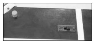
❑ Using the switch cover as a template, cut an opening in the side of the fuselage to mount the switch in. It should be on the left side of the fuselage. Drill two 1/16" holes for the switch mounting screws and install the switch.
