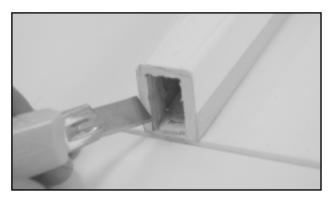
□ Carefully cut a hole with hobby knife at the tail as the elevator pushrod exit.
