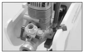
❑ Set the engine on the mount and adjust the beams, if necessary, so that they are almost touching both sides of the engine crankcase and are centered in relation to the engine mount back plate. Now position the engine so that the front of the thrust washer is approximately 4" from the fire wall. Note: you will probably have to trim away the fuselage side for needle valve clearance.
