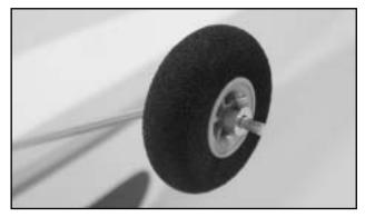
□ Install the wheels onto the main gear using the suplied wheel collars and 3 x 5mm screw. Make sure the wheel rotates freely.
