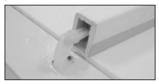
□ Mount the control horn with 2 x 12mm screws. Insert the elevator pushrod with clevis threaded on. Cut a small piece of silicone and slide it onto the clevis. Then, snap the clevis on the outmost hole of control horn.
