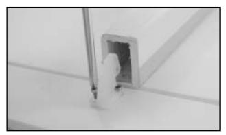
□ Use control horn as template and drill 5/64" holes with the contorl horn in line with the hinge line of elevator and right at the pushrod exit.
