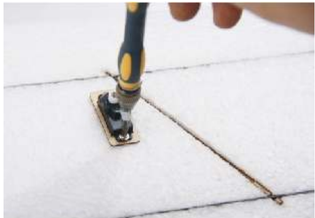
10. Fix the servo onto to the sevo mount by using 2pcs self-tapping screw which included into the servo parts bag.
