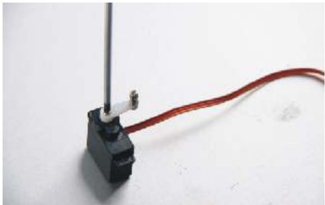
7. Install the pushrod connector onto the first hole of the servo arm , and then install the servo arm onto the servo , pls make sure the servo arm is in the neutral position.
