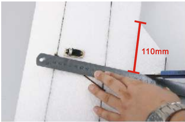
11. Pls cut a slot by using knife as the picture shown , it's convenient for installing the control horn.
