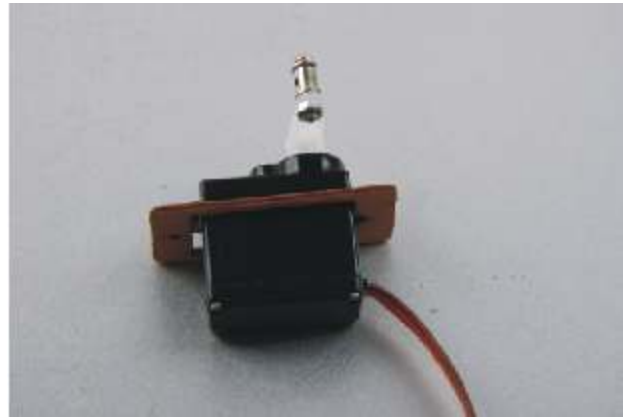
8. Install the servo into the servo mount.
