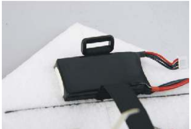
19. Fix the ESC by using the plastic band , as the picture shown.
