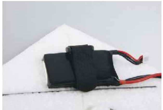
20. Fix the battery by using velcro.
