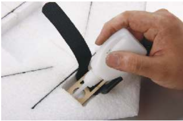
5. Glue the battery velcro by using CA.
