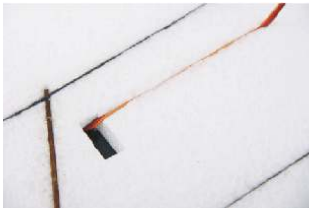
18. As the picture shown , using a knife to open a servo wire slot , so that the wire can easily reach to the equipment compartment , and then put the servo wire into the pre-cut slot.
