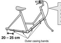
There should be enough slack so that the cable is not pulled too much when the handlebars are turned.
