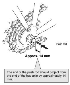
2. While pushing the main bell crank unit onto the hub axle, align the serrations inside the main bell crank unit with the flange nut, and then push the main bell crank unit on until it touches the end of the hub axle. In this position, tighten the main unit installation bolt onto the hub axle.
