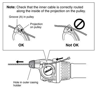
2) Hook the inner cable into groove (B) in the pulley, and pull the inner cable so that the inner cable drum fits into the hole (B) in the pulley. After this, insert the outer casing into the outer casing holder.
